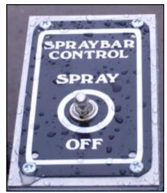
**1 Foot Sectioned Spray Nozzle Control** Allows on/off control of any 1 foot section of the spray bar. Gives outstanding flexibility in selecting spray patterns for your changing needs.
