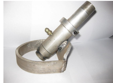
Part # A10020453(4" alum "U" swivel 1/4 x 53°) Part # A10020458(4" steel "U" swivel 1/4 x 53°) "U" shaped shoe 4" wide with built-in swivel constructed of lightweight aluminum for less operator fatigue and ease of operation. Grease fitting on swivel for long life. All aluminum construction with 3/4" NPT
