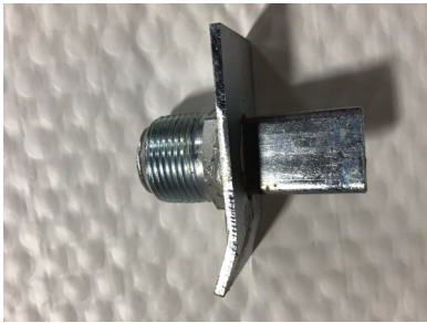
Part # 204095 5/16 flat steel 1/4 straight 5/16" wide flat nozzle typically used for applying sealer into sawed cuts in concrete or asphalt. Steel construction with 3/4" NPT Threads.
