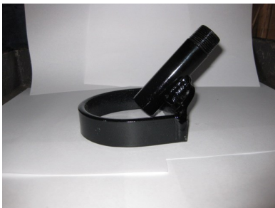
Part # W10018004 (4" steel "U" 1/4 x 53°) "U" shaped shoe 4" wide gives you a medium width over-band and eliminates the need for a second squeegee operation. Steel construction with 3/4" NPT Threads.
