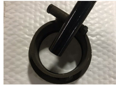
Part # 204053 (4" steel "O" 1/4 ) "O" shaped shoe 4" wide gives you a narrow over-band and eliminates the need for a second squeegee operation. Steel construction with vertical swivel with 3/4" NPT Threads.
