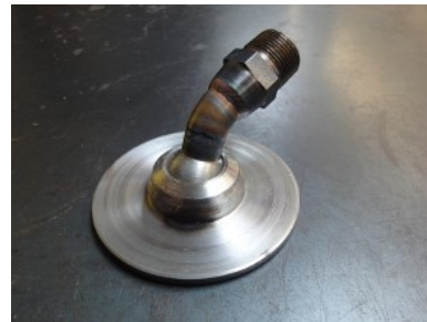
Part # P10017455(4" stainless steel Disk 3/4" Adjustable) Adjustable approach angle for customized operator comfort. 4" circular disk with turned up edge gives you a medium width over-band and eliminates the need for a second squeegee operation. Steel construc- tion with 3/4" NPT threads.
